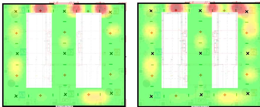
(a) Heat map of the median values on all reference positions. (b) Heat map of compass error mean values.
