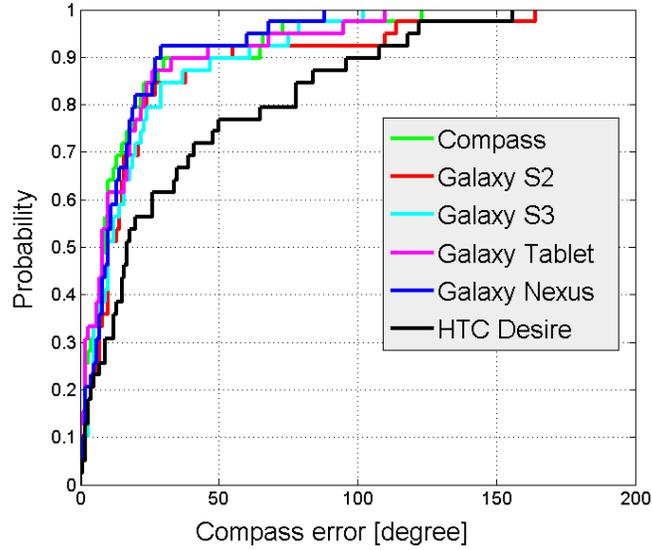
**Fig. 3.** Cumulative distribution function of the error values on several mobile devices.
