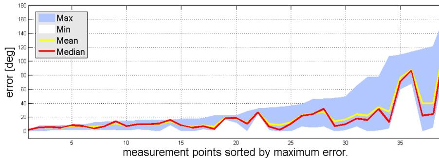
**Fig. 4.** Measured error values of all mobile devices at 39 reference points. The graph is ordered by the maxima that was captured for each position.
